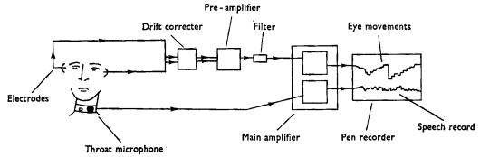
FIGURE 1 Apparatus.
