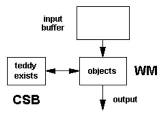
Figure 6 - Alternative architecture with the Current State Buffer (CSB) separate from the input buffer.
